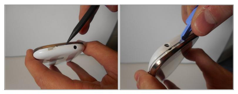
• Locate the small indent in the top of the device and use your nails or a spudger to separate the cover from the mid-frame.
