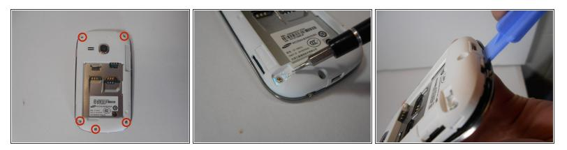
• Remove the five 3mm screws along the top and bottom edges of the device with the Philips #00 screwdriver.
