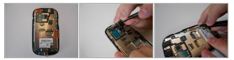
Locate the two ribbon cable connections on the motherboard. GENTLY use the pointed end of the spudger to disconnect the cables. Lift the motherboard out of the phone.
