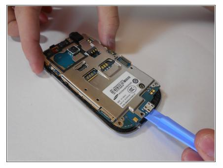
Using your fingers or a plastic opening tool, carefully lift the motherboard assembly from the phone.
