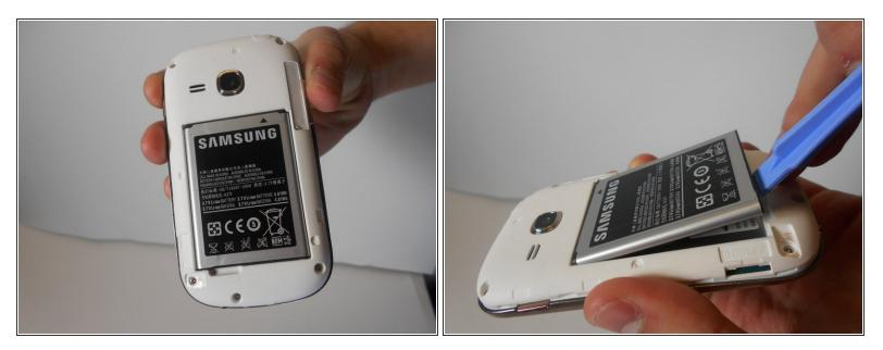
Locate the indent on the bottom left corner of the battery compartment. Use your fingers or the plastic opening tool to lift the battery from the device.
