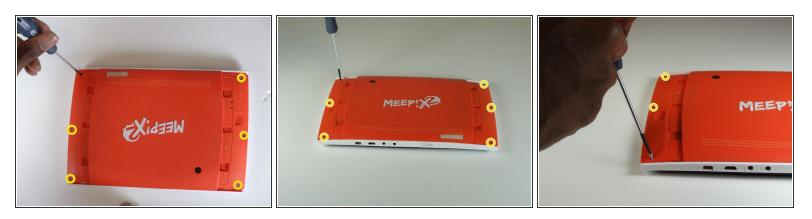
You can remove the rear casing by unscrewing all six phillips #00(3.5mm x 4.5mm)screws from the left and right side of the device.
