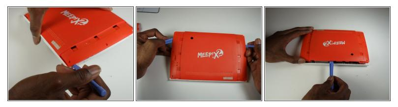
• Use the plastic opening tools to undo the clips around the edges of the device.
