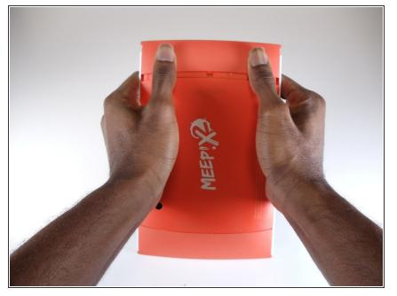
Remove the orange covers from the left and right sides of the device by sliding up against the tabs.
