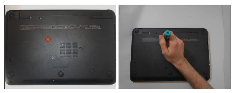
There is one screw holding the DVD±RW Drive in place. Use the #00 screwdriver to remove the screw.
