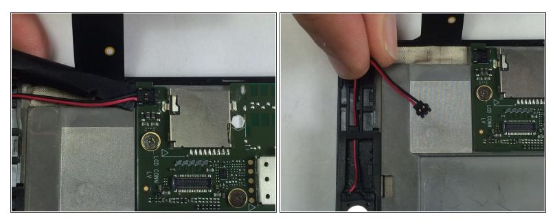
Disconnect the speaker wire from the motherboard by prying the connector upwards with the spudger.
