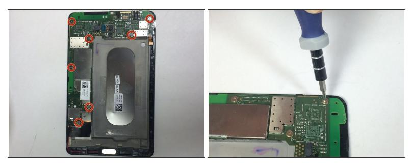
• Remove all 8 of the 2.1mm Phillips head screws from the motherboard.
