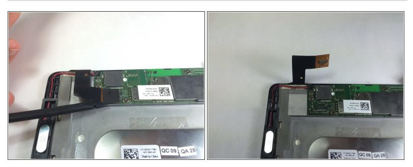
• Use a spudger to remove the ribbon cable that is around the speaker wire.
