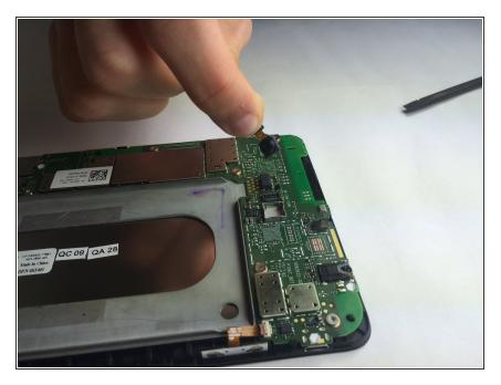
• Remove the camera from the device.
