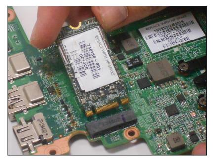
Remove the hard drive by pulling the device from the black slot.
