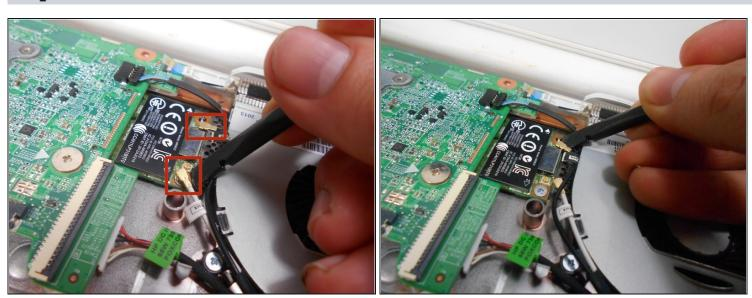
Using a spudger, remove the white and black cables from the card.
