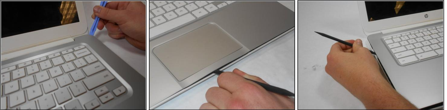
**⚠ Warning!** When prying open a laptop it could require some force, but it also has fragile connectors underneath. Use caution so as to avoid breaking these connectors.
