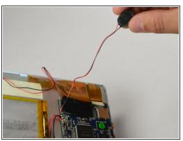
Remove two strips of tape: One holding down the wires and the other holding down the internal speaker.
