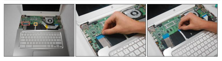
A Warning! Handle the flaps and ribbon cables with care to prevent damage.
