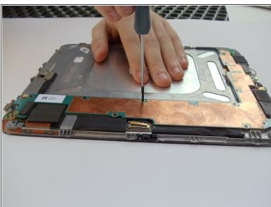
Remove the ten 2 mm black screws from the edges of the system board with a Phillips #00 screwdriver.
