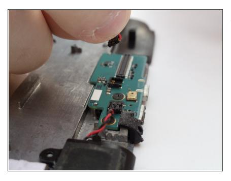
Pull up on the connection to disconnect the speakers.
