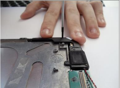
• Remove the seven 2 mm black screws connecting the speakers using the Phillips #00 screwdriver.
