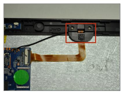
• The camera head is located on the upper middle section of the device, close to the battery.
