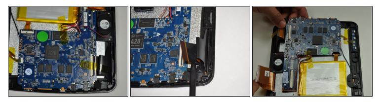
• Gently lift the motherboard up and out of the device.
