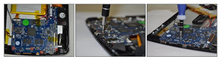
• Using the Phillips #000 screwdriver, remove the four 5 mm screws located in the picture by rotating the screw counter-clockwise.
