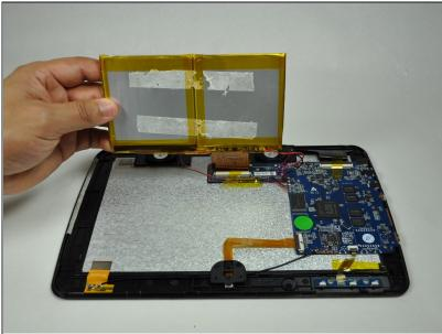
• Gently lift the battery up and out of the device.
