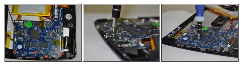
Using the Phillips #000 screwdriver, remove the four 5 mm screws located in the picture by rotating the screw counter-clockwise.
