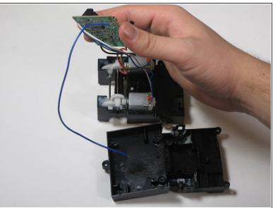
• Lift the circuit board from the plastic casing and flip it over to expose its underside where the wires are connected.
