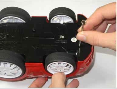
• Flip the car over and remove the four 5mm Phillips #0 screws that hold the shell to the car chassis.
