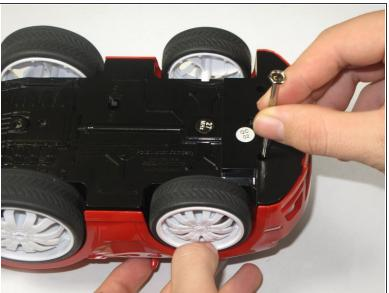
Flip the car over and remove the four 5mm Phillips #0 screws that hold the shell to the car chassis.
