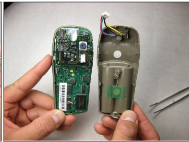
With tweezers (or your fingernails), carefully disconnect the wires between the PC input and the motherboard.
