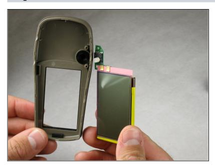
• Insert the new LCD screen in the device.
