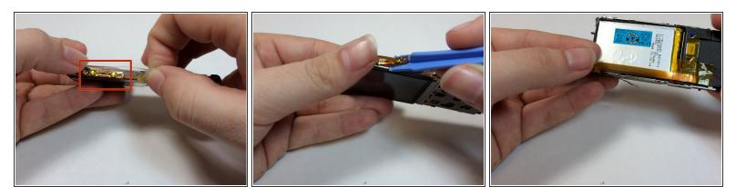
• Use a prying tool to pry under the volume control module.
