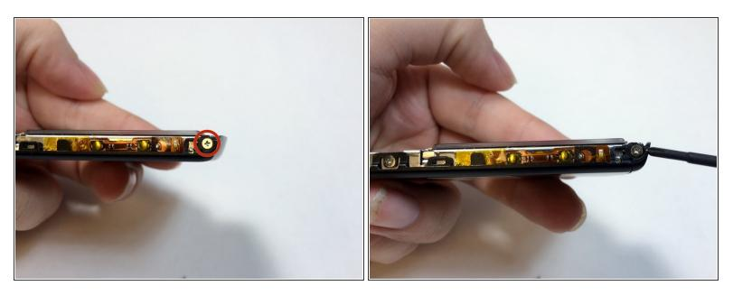
• Remove the two 2.8 mm phillips screws located on either side of the device near the top.
