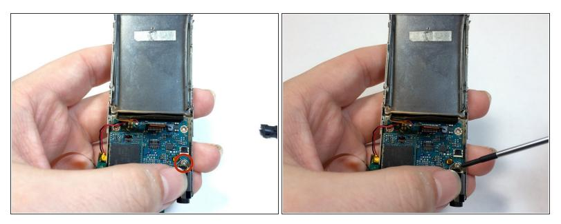
Peel back the ribbon for the audio jack and remove the 1.8mm silver Phillips screw.
