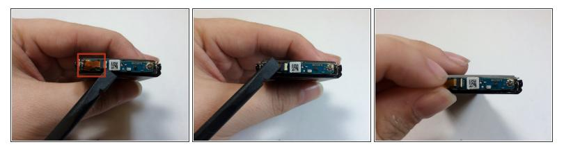
• Use the flat end of the spudger to flip up the retaining flap for the bluetooth module.
