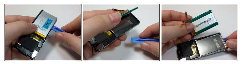
• Insert a plastic opening tool under the battery and lift up to remove it.
