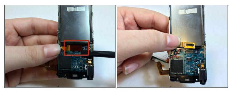
Use the prying tool to remove the LCD ribbon wire.
