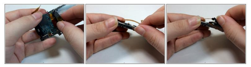
• Remove the plastic bracket by pushing up with your thumb to expose the display connection.
