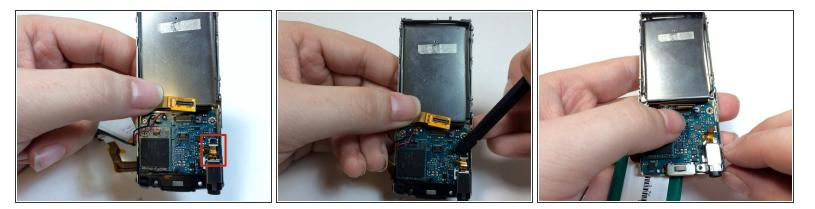
• Use the flat end of a spudger to flip up the retaining flap on the audio jack module.
