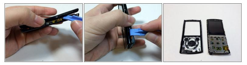
Using a plastic opening tool, work your way around the edges of the device, carefully prying off the front panel.
