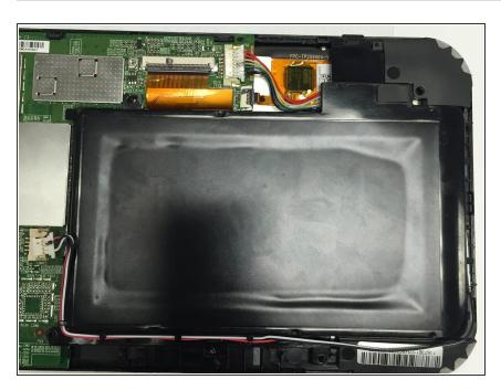
Install the new battery into your device, re-install the speakers, and perform the first six steps in reverse.
