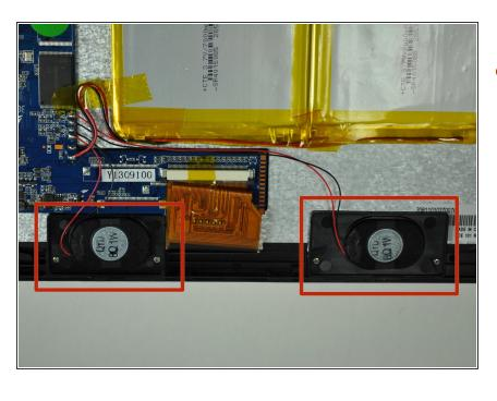
The speakers are located on the bottom of the device, below the battery and adjacent to the motherboard.
