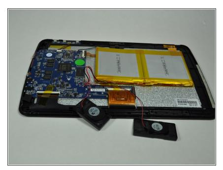
Gently lift the speakers up and out of the device.
