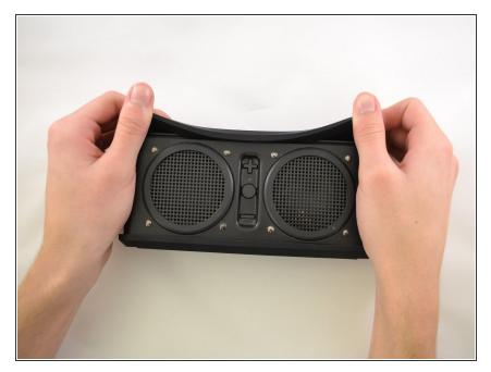
Starting with the corners, gently pull the rubber cover off of the device.
