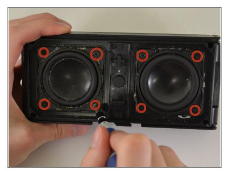
Using a #000 Philips Screwdriver, unscrew the four 8 mm Philips screws from each corner of both speakers (eight 8 mm Philips screws total).
