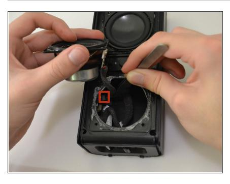
Firmly pull on the end of ribbon cable to disconnect the speaker from the motherboard.
