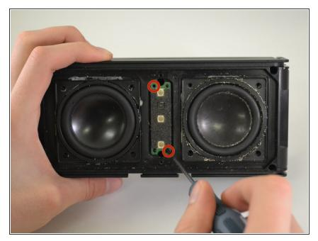
Using a Phillips #00 Precision Screwdriver, unscrew two 6 mm screws from the button motherboard.
