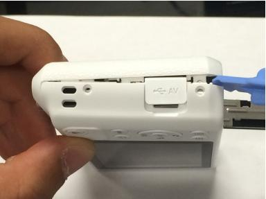
Using the spudger, and plastic opening tool open the casing of camera.
