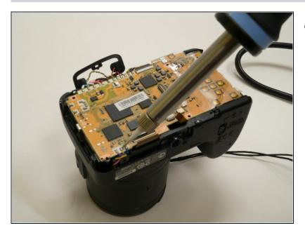
Unsolder the wires on the bottom end of the motherboard.
