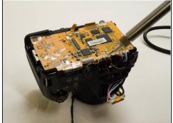
• Unsolder all the wires that are on the top of the motherboard near the flash component.
