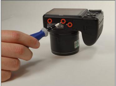
• Remove three 5 mm Phillips #000 screws on the bottom end of the camera.
