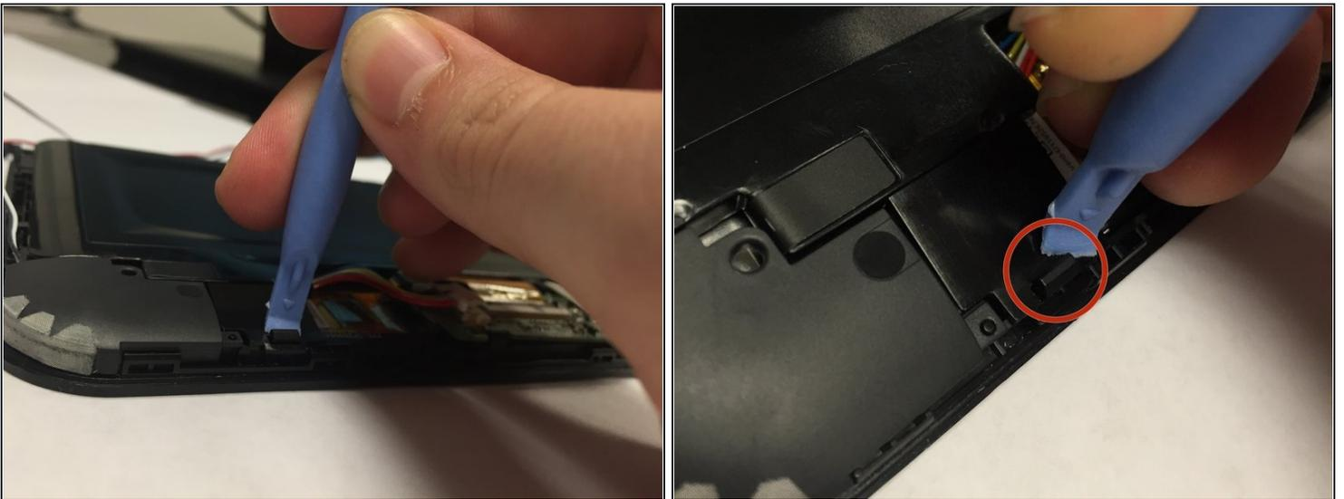
ⓘ The battery has one clip you will need to remove. The clip is located at the bottom right corner of the battery just above the right speaker. The speakers and wires are not secured to the battery, they may fall off.
