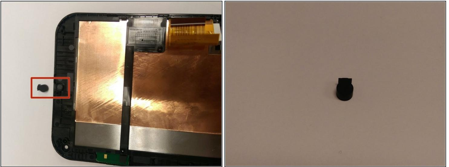
ⓘ The screen has a rubber device used to support the volume control switch.
