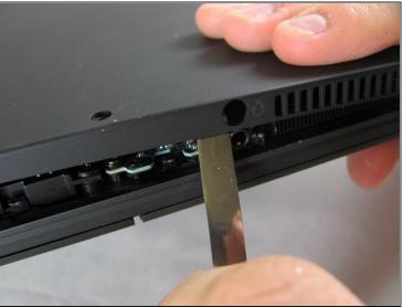
• Use the Plastic Opening Tools or Metal Spudger to carefully loosen back cover from the body of the computer.
