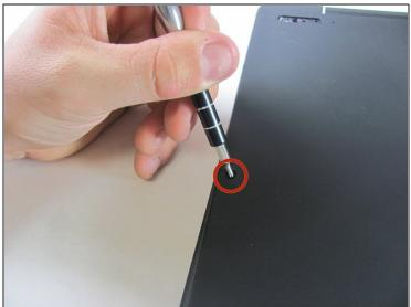
• Starting with the laptop top-down, locate and remove the twelve 1mm Phillips #0 screws securing the back cover to the main body of the computer.
