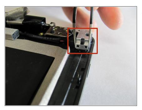
Use tweezers to carefully remove the charger port cover.
