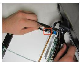
• Use tweezers to carefully separate the two connections of the strip from screen back panel.
