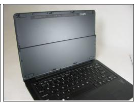
Unlock the screen and lift the corner. Carefully turn it over until it faces away from the keyboard.
