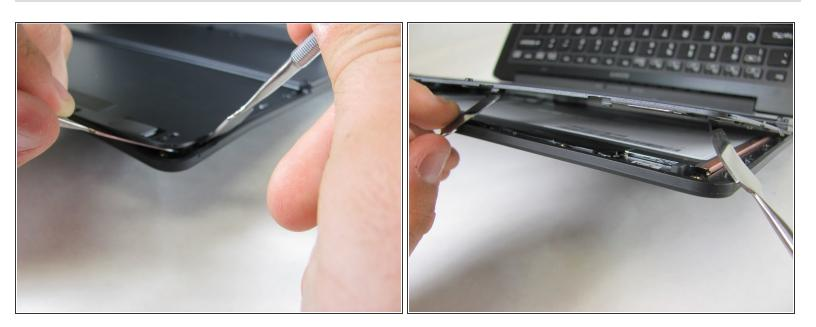
Use the Metal Spudger Set to carefully separate screen from backing. Be sure to keep the grey panel flush with the screen front.
