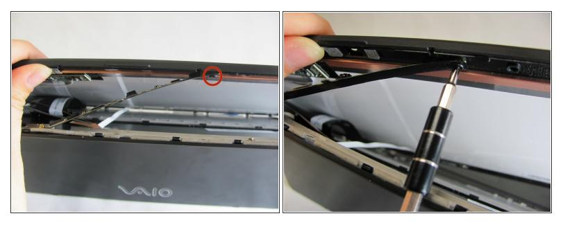
Remove the single 1mm Phillips #0 screw that is connecting the screen and the device.
