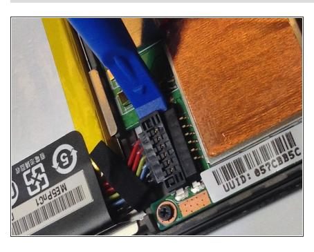
Insert the plastic opening tool under the side edge of the battery connector, and gently pry upward to disconnect it.
