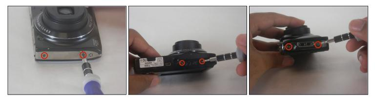
Unscrew the six 3.5mm Philips head from the outer casing.
