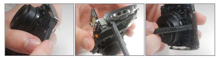
• Pry the center casing off the camera. This is best done by separating the top and side sections individually.
