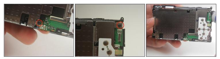
• Unscrew the two 3.5 mm Phillips head screws in the metal plate.
