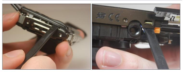
• Pry the back half of the casing from the camera.
