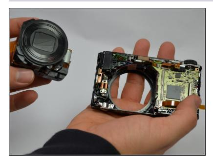
• The lens can now be removed from the camera.
