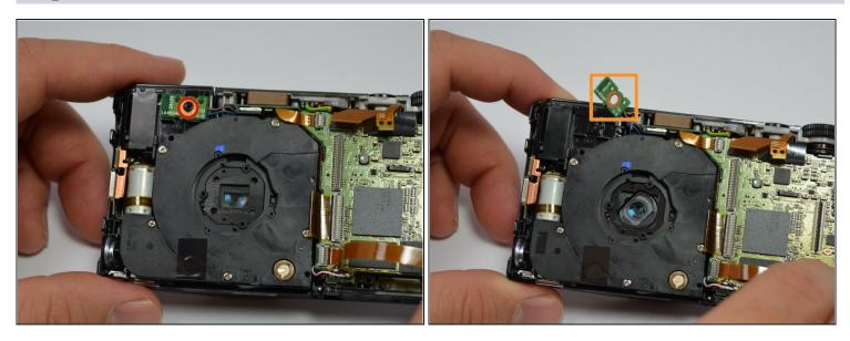
• Remove the 3.5 mm screw holding down the Wi-Fi card.
