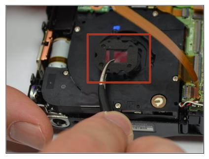
• Using <u>tweezers</u>, remove the lens cover from the lens.
