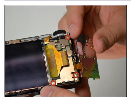
• Remove the three 4 mm screws with a #00 Phillips screwdriver.
