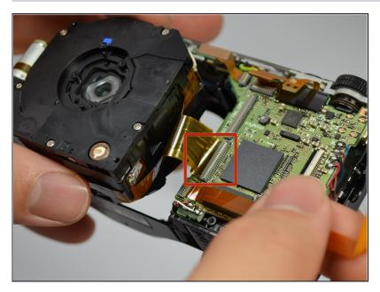
Detach the ribbon cable connecting the lens unit and circuit board.
