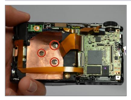
Remove the three 4 mm screws using a #00 Phillips screwdriver.
