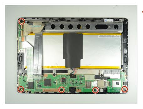
Remove the five screws using a Phillips #00 screwdriver.
