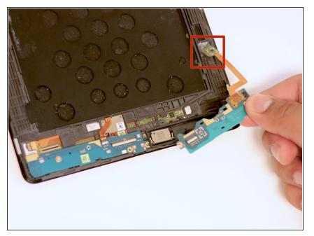
The daughterboard has an orange ribbon cable that is adhered to the device. Gently pull the ribbon up and remove the daughtboard.
