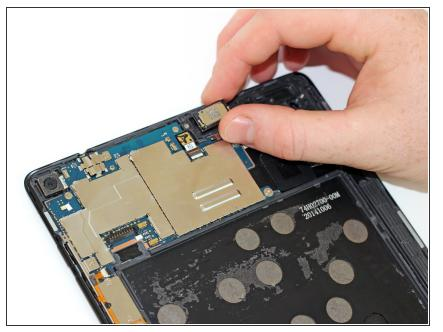
Use a spudger or your fingers to remove the first speaker. The speaker may be heavily glued in and require heat to lift. Be careful as you can pull the speaker apart.
