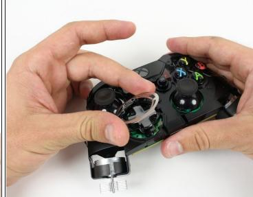
• Pry off the metal frame around the D-Pad.
