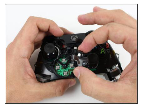
• Lift the D-Pad out of its housing.
