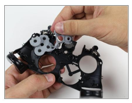
Remove the rubber backing to the buttons.
