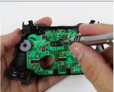
Remove the six T6 Torx screws located on the bottom motherboard.
