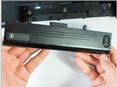
Remove the battery using two hands and pull it away from the computer.
