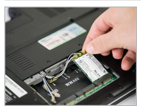
Lift the card out at an angle and carefully remove it.
