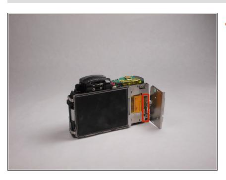
Carefully remove the ribbon connecting the control panel to the camera. The latch can be removed by sliding it down and pulling the ribbon down.
