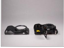
Separate the case using the plastic prying tool. This can be done by placing the tool in the position that is shown and in the position on the left side of the camera.
