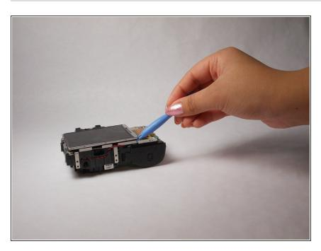
Using a prying tool, carefully lift up the LCD screen but do NOT pull it off.
