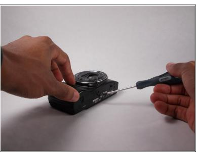
Remove the four (3.20 mm) Phillips #00 screws at the bottom of the device.
