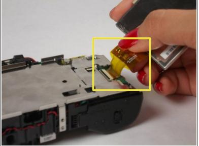
While the LCD screen is loose and unattached, there is a latch that is holding the ribbon in place.
