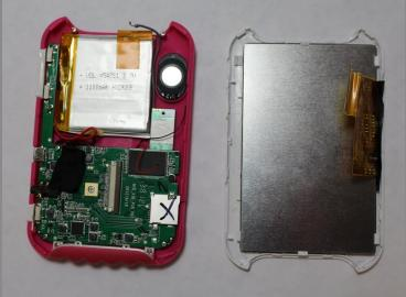
• Disconnect the LCD cable from the motherboard by pressing together the two sides of the clamp to separate the device into two.
