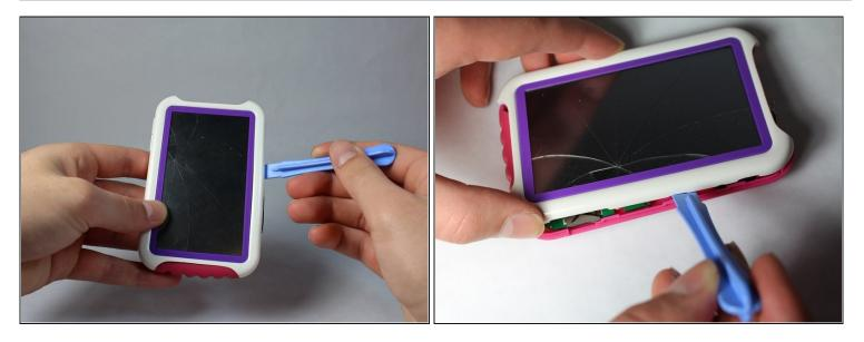
Use a spudger to pry open the case. Do this on the long side of the case. This will reveal the inside.
