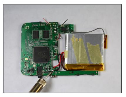
Unsolder the gray, black, and red wires from the motherboard to release the battery.
