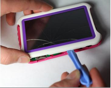
Use the opening tool to pry open the device case.
