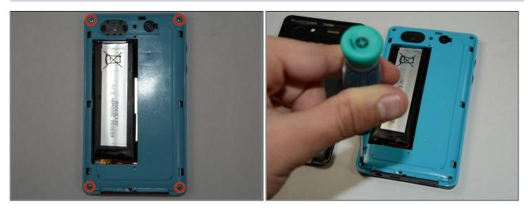
• To remove the battery, make sure the four 5mm Philips screws on each side of your device is open using the Philips#1 Screwdriver.
