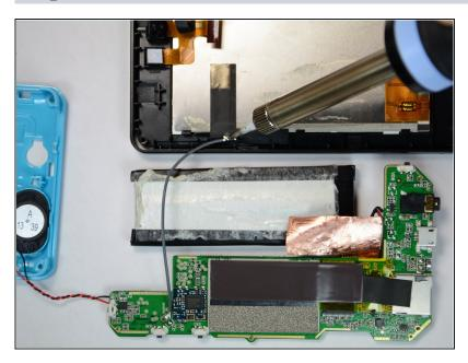
• Use the soldering tool to remove the wire that is attached to the screen & the motherboard.
