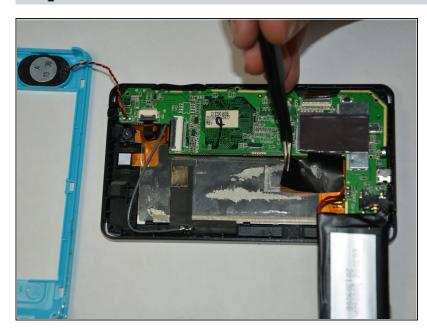
• Use <u>tweezers</u> to remove the black tape that is attached to the motherboard.
