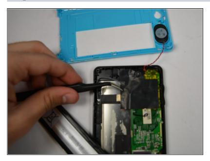
• Remove the plastic cover that is covering the camera area.
