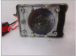
Remove the old blades by pulling them away from the gears and motor.
