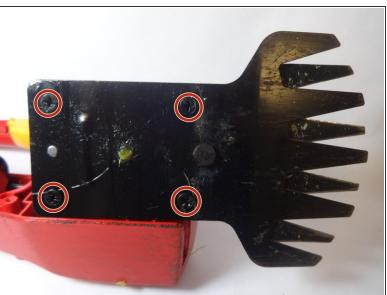
Use the Phillips #2 screwdriver to remove the four 10.0 mm screws on the bottom of the blades.
