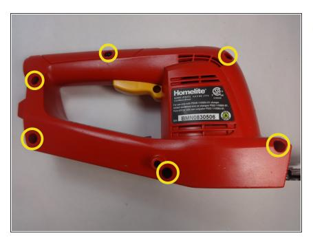
Remove the six 15.0 mm screws from the body of the device with a Phillips #2 screwdriver.
