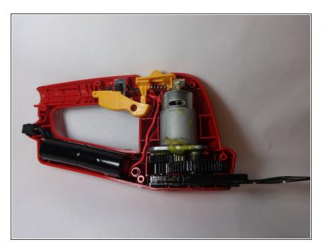
Remove the face plate by lifting it away from the other half of the device. This will expose the interior.
