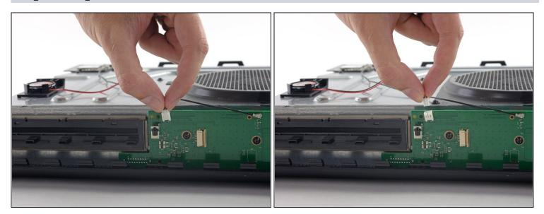
• Gently pull up on the speaker cable connector to disconnect it from the front panel board.
