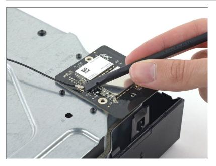
Use the flat end of a spudger to disconnect the Wi-Fi antenna cable from its socket on the Wi-Fi board.
