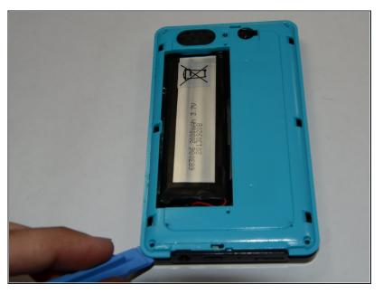
After you remove your four 5mm Philips screws use your plastic opening tool to help you open the plastic cover of your device.
