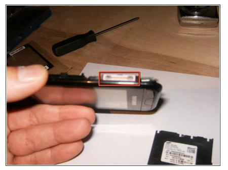
• You also must remove the camera shutter and extra media buttons cable. It is glued to the side of the frame and the plactice tool with a slight tuck will loosen the adhesive strip underneath.
