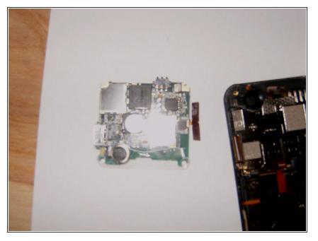
Remove both of these wires. The LCD one is a push-on connector and the Digitizer has a small retaining clip. Be careful that you do not break it while trying to open it. This is where patience will pay off. Gently remove the motherboard ensuring that all the connections are loose.
