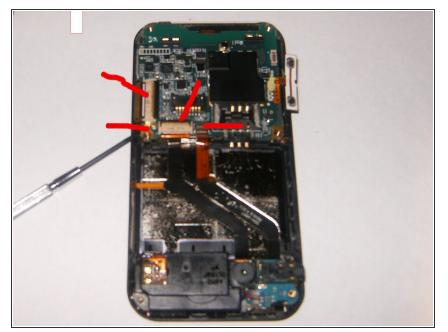
• You will now see 4 connectors on the motherboard that need to be removed. You unhook these by carefully lifting up the latch lock (the black bar on the connector) and then slide the cable out. The antenna cable does not have a latch, you remove it by just lifting it up.
