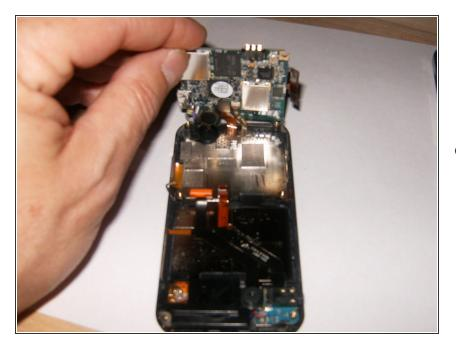
Once the cables on top of the motherboard have been disconnected, tilt the mother board gently up and to the back. Be careful, there are 2 more ribbon cables connected on the underside. The broader cable is for the LCD and the smaller one is the digitizer cable.
