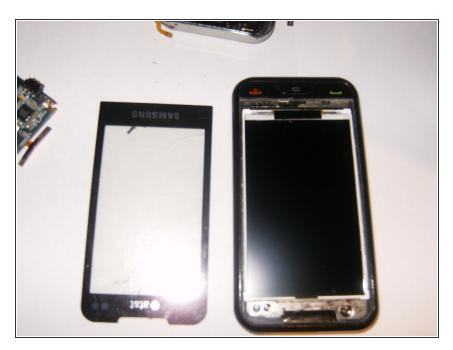
• Turn the phone over so that the LCD is facing upwards. I used a small plastic tool to loosen the digitizer from the frame. This will take patience and plenty of repetitious scraping around the outline of the digitizer. Do not force it since it might break your old digitizer. Of course, if it is already going to be replaced it might not matter.
