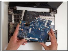
Carefully pick up the Mother board and disconnect the Battery cable.
