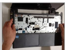
Carefully separate the upper cover and remove it.
