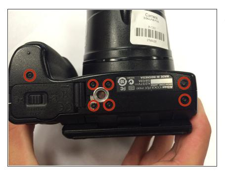
• Flip the camera upside down and remove the seven marked screws.
