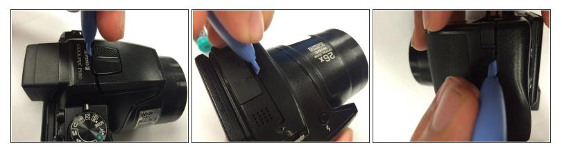
• Use a plastic iFixit opening tool to gently loosen the top and sides of the camera.
