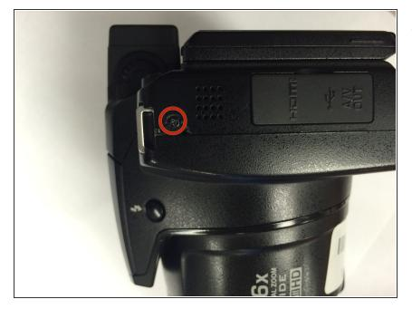
On the right side of the camera, remove the first visible screw above the HDMI and A/V OUT cover.
