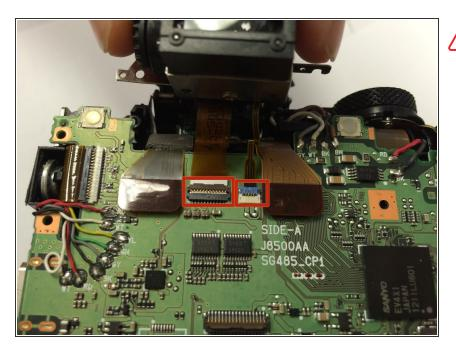
Carefully detach the two ribbon cables and detach the viewfinder.
