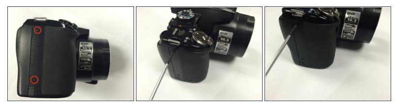
On the left side of the camera, use a Phillips #00 Precision Screwdriver to remove the two marked screws.
