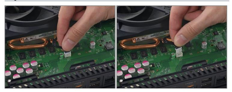
• Disconnect the fan cable from the motherboard.
