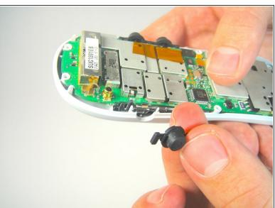
Lift and remove buttons by hand
