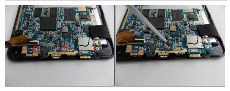
• Use the T4 Torx screwdriver to remove the 4.0 mm T4 Torx screws.
