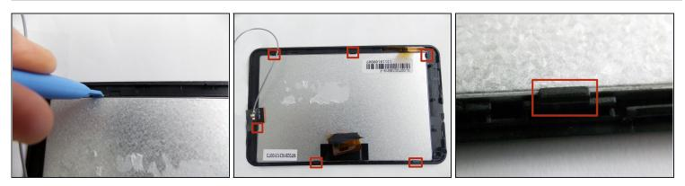
• Insert the plastic opening tool between the screen and the case to release the clasps holding the screen.
