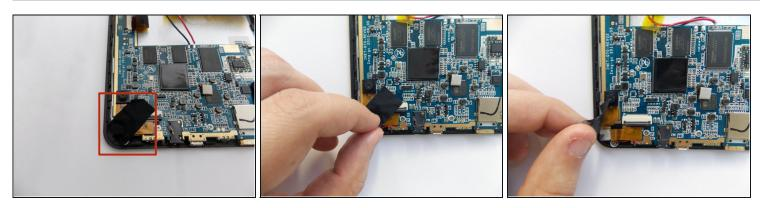
• Remove the black tape covering the cameras power cable.
