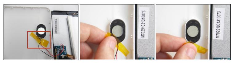
• Remove the tape holding the speaker in its socket.
