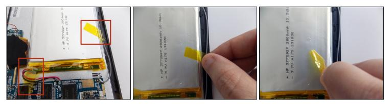
• Remove the tape holding the battery in place.
