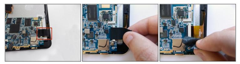
• Remove the black tape covering one of the screen power cables.
