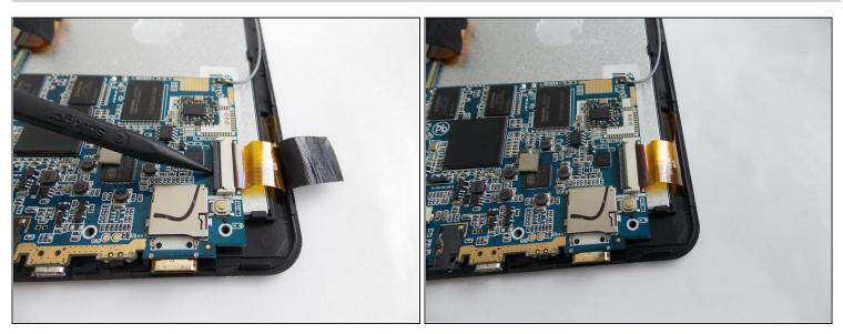
• Use the spudger tool to pry the ZIF connector upwards so that it releases the power cable.
