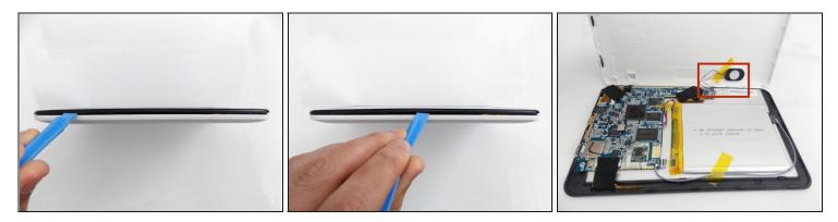
• With the plastic opening tool in the opening between the two sides of the case, slide the tool along the tablet's border to separate the two sides completely.
