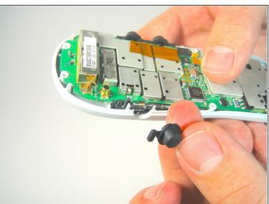
Lift and remove buttons by hand
