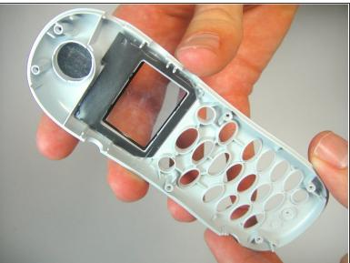
Once the motherboard, speaker, and keypad have been removed you should have the front cover by itself
