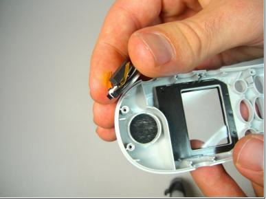
Use the iFixit opening tool to lift the speaker off the front cover.
