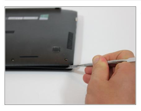
Use a plastic or metal spudger to separate the keyboard from the back panel and lift the keyboard out of place.
