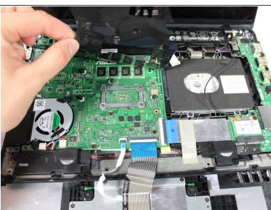
Use the spudger to lift up and remove the black plastic covering.
