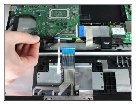
Remove thinner white strip by first flipping up black piece at the top of the strip with the tweezers and then pulling it out.
