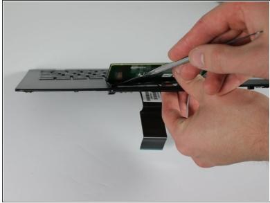
• Use metal spudger to get in between mouse pad and keyboard and lift off.
