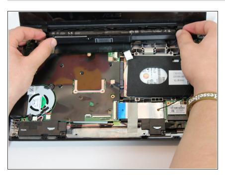
Slide the battery up and out.
